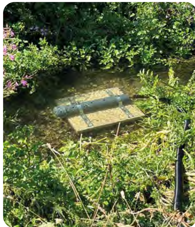
Sensor mounted horizontally on riverbed due to shallow water
