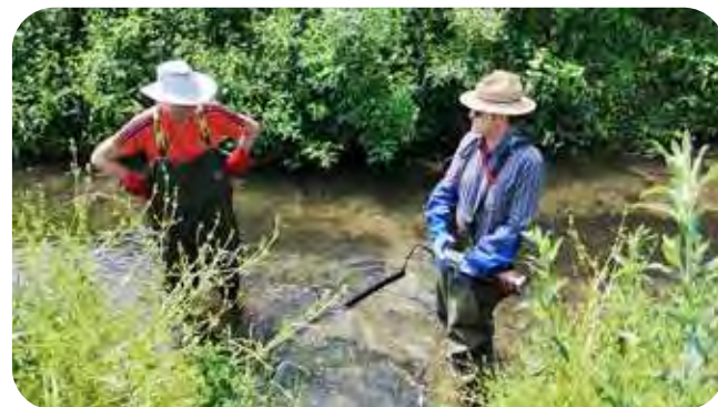
Cleaning the sensors on a sonde.
