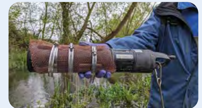
Protective copper mesh around a sonde to prevent fouling by sediment and algae
